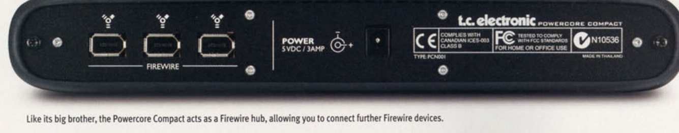
Like its big brother, the Powercore Compact acts as a Firewire hub, allowing you to connect further Firewire devices.
